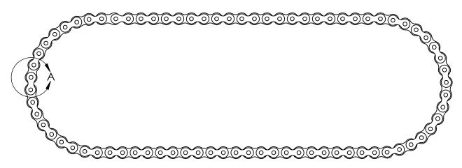
SINGLE ROW SINGLE LOOP 25 SERIES CHAIN 78 TOTAL LINKS 78 OUTSIDE PLATES 78 INSIDE PLATES 78 PINS
